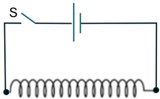
State and explain what, if anything, will happen to the separation of the coils of the solenoid when the switch  $S$  is closed. [2]
